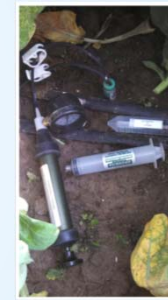
Fig. 4. Vacuum pump and syringe to collect soil solution.
