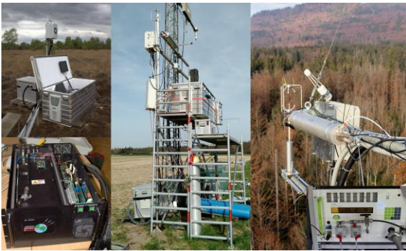
Fig. 1: Campaign setups – Left: Bourtangier Moor peatland site (BM) with QCL; Middle: cropland in Braunschweig (TI) with TRANC; Right: Bavarian Forest National Park (BF) with TRANC and CLD.
